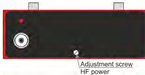
Fig. 7: Adjustment of stator antenna
