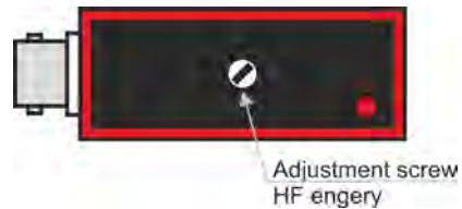
Fig. 7: Adjustment of stator antenna
