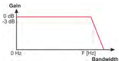
Fig. 6: Gain bandwidth characteristic
