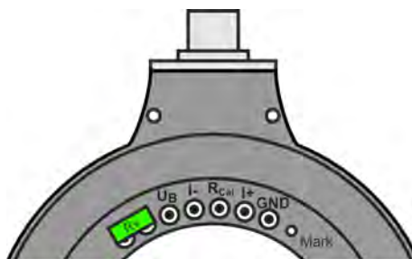
Fig. 5: SV_2Lg_PCM16, pin assignment
